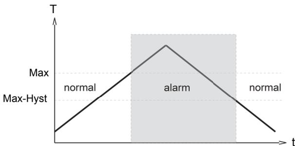
A switchover delay time ( $t_{DS}$ ) can be applied to the switchover to the alarm state. Equally, one switch-back delay time ( $t_{DR}$ ) of several can be applied to switching back to the normal state.
