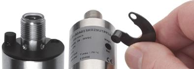
If the contact time is longer or shorter than this, no programming takes place (protection against external magnetic fields). Immediately after programming, the switching output goes into the normal state (see below).
