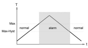
A switchover delay time  $(t_{DS})$  can be applied to the switchover to the alarm state. Equally, one switch-back delay time  $(t_{DR})$  of several can be applied to switching back to the normal state.
