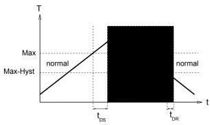
In the non-inverted (standard) model, while in the normal state the switching output is at the level of the supply voltage; in the alarm state it is at 0 V, so that a wire break would also display as an alarm state at the signal receiver. Optionally, an inverted switching output can also be provided, i.e. in the normal state the output is at 0 V, and in the alarm state it is at the level of the supply voltage.
