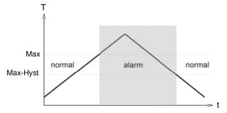
A switchover delay time  $(t_{\text{DS}})$  can be applied to the switchover to the alarm state. Equally, one switch-back delay time  $(t_{\text{DR}})$  of several can be applied to switching back to the normal state.
