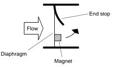
There is a plastic-coated magnet on the diaphragm. When there is a deflection, its magnetic field changes, and this is detected by a sensor outside the area of flow.
